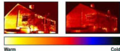
Air leakage affects the thermal performance of a home, and can account for 30% or more of your home's utility bill. Oak Ridge will conduct blower door and duct testing to determine the natural infiltration rate of the house and duct system. Uncontrolled air leakage can result in high fuel bills and moisture damage.
