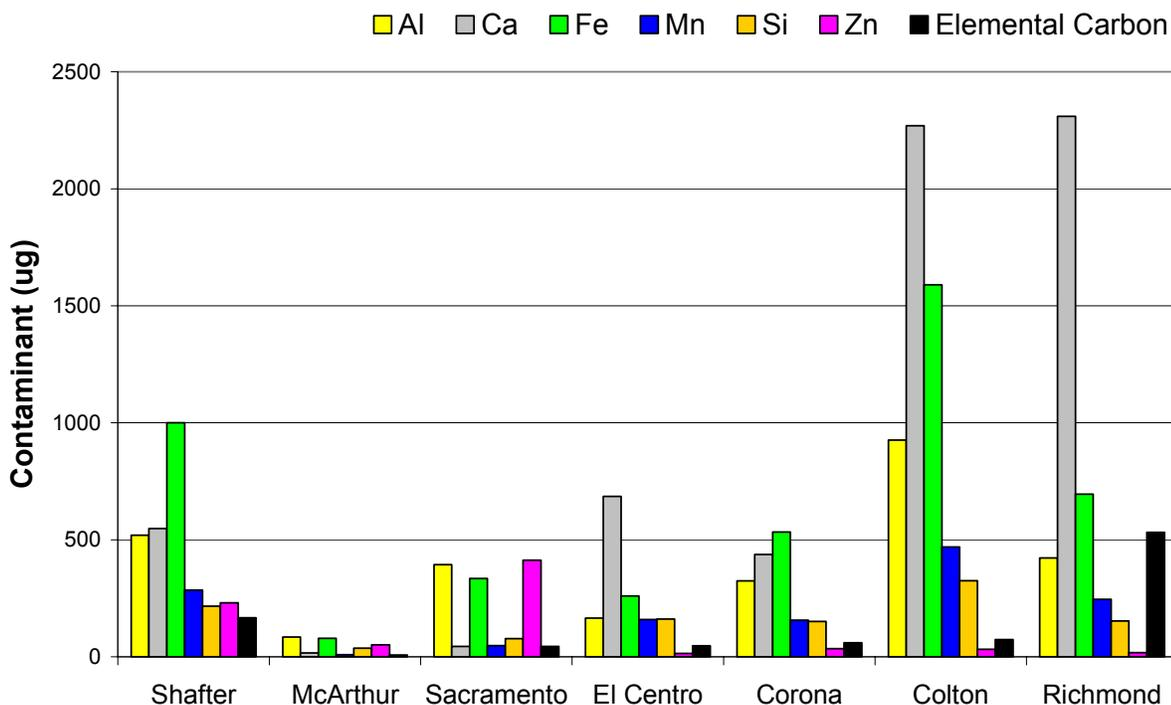
Figure 1. Major elemental contaminants measured on roof samples pulled from CA weathering sites.
