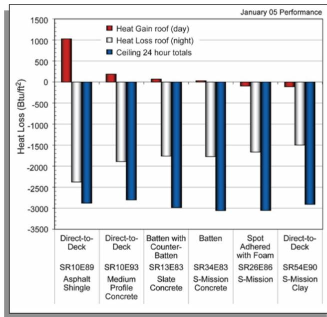
Figure 3. Heat flow measured for all tile and shingle roofs during the month of JAN 05.
