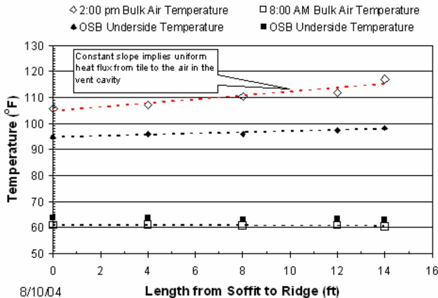
Figure 3. Bulk air and deck temperature measured in the inclined air channel of the clay tile roof.
