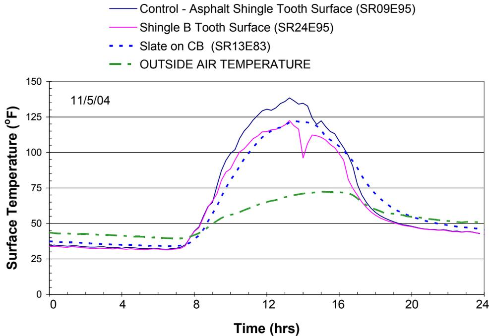
Figure 2. Surface temperatures measured on the steep-slope attic assembly at ORNL
