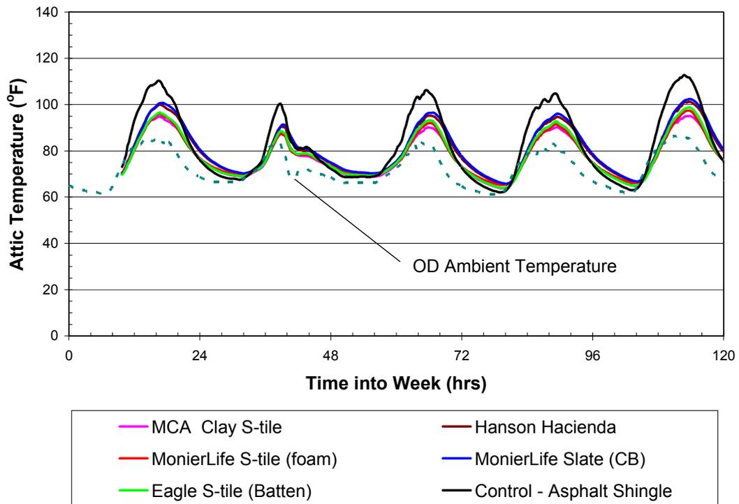
Figure 3. Attic air temperature measured under each of the tile roofs being field tested at ORNL.
