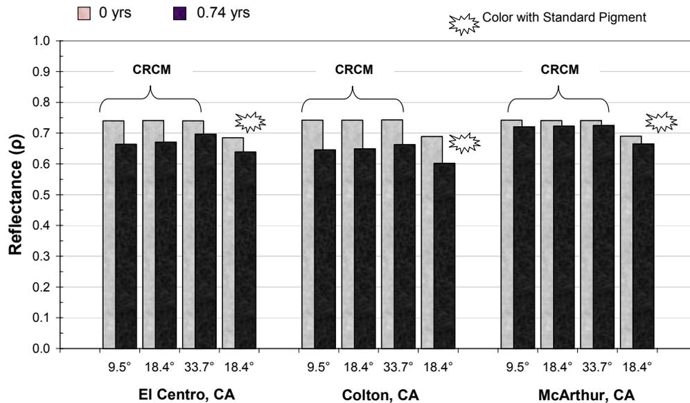
Figure 2. White painted polyvinylidene fluoride metals with and without CRCMs. The slopes of 9.5°, 18.4° and 33.7° represent respective exposure settings of 2-in, 4-in and 8-in of rise per 12-in of run.
