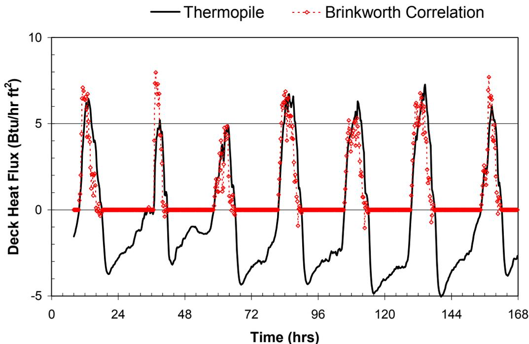
Figure 2. Comparison of heat flow measured by heat flux transducer in OSB deck against heat transfer correlation by Brinkworth (2000).
