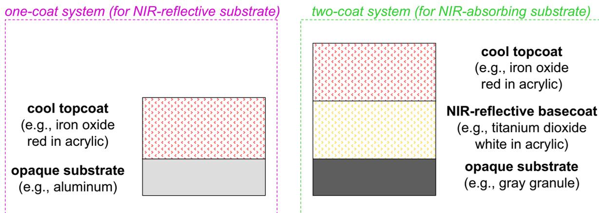
**Figure 1. Schematics of one-coat (substrate + topcoat) and two-coat (substrate + basecoat + topcoat) systems. The one-coat system can also be applied over an NIR-absorbing substrate if the topcoat has at least moderate NIR backscattering and is sufficiently thick.**
