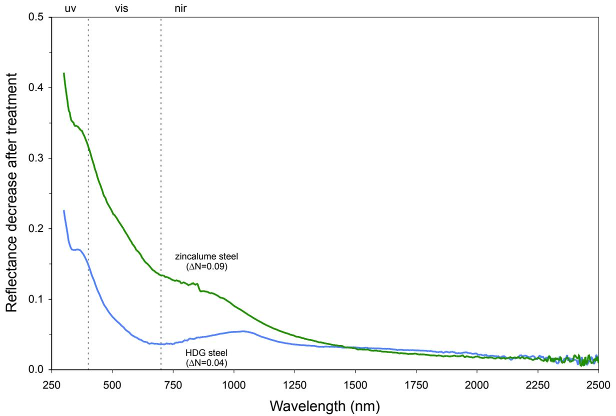
**Figure 4. Decreases in spectral reflectance induced by treating ZINCALUME<sup>®</sup> and hot-dipped galvanized (HDG) steels.**
