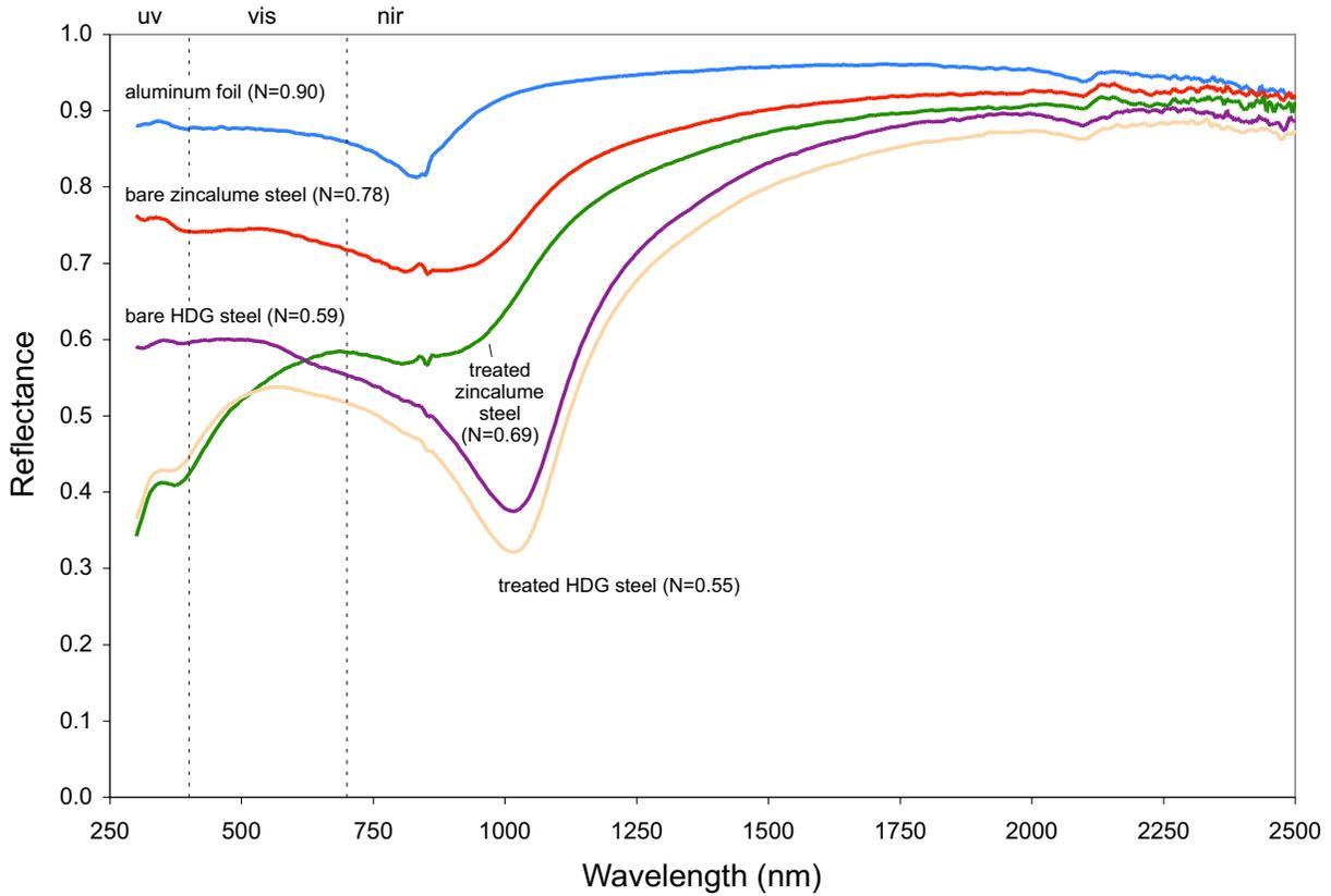
**Figure 3. Solar spectral reflectances and NIR reflectances (N) of five uncoated, metallic substrates: aluminum foil, bare and treated ZINCALUME<sup>®</sup> steels, and bare and treated hot-dipped galvanized (HDG) steels.**
