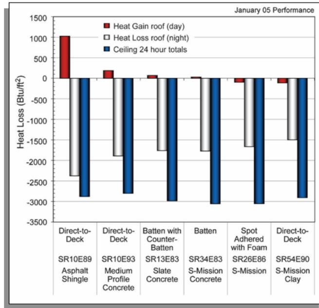
Figure 1. Heat flow measured for all tile and shingle roofs during the month of January 05.
