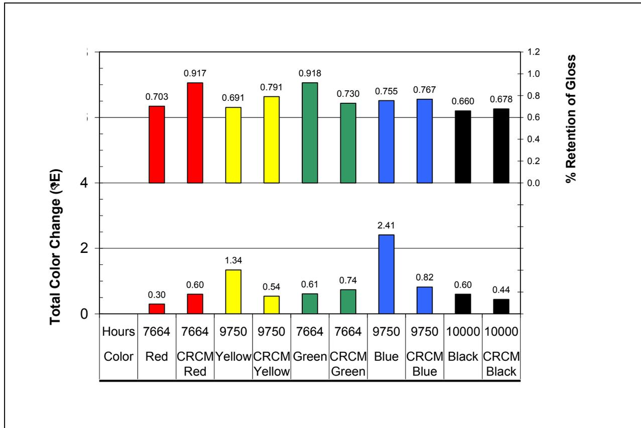
Figure 2. The total color change and the retention of gloss for masstones tested under fluorescent UV light using ASTM G154 protocol. (Data courtesy of BASF).
