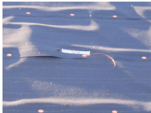
Figure 1. Thermocouple used for measuring metal roof temperature.
