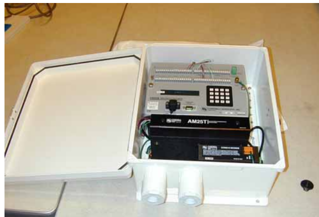
Fig. 2. Campbell Scientific CR23X data logger for demo home.
