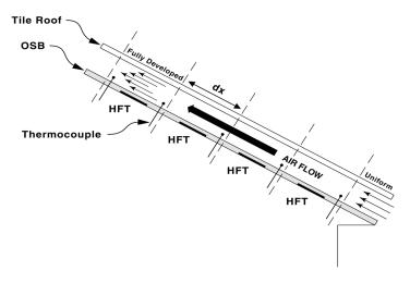
Fig. 3. Cross-section showing measurement scheme to infer airflow in vent gap.
