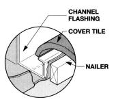
discussion however, we decided to use a parapet partition with channel flashing (see figure) between each test roofs to eliminate any effects of transverse airflow from one test roof to another.
