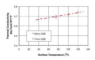
Figure 1. Thermal conductivity measures made for OSB.
